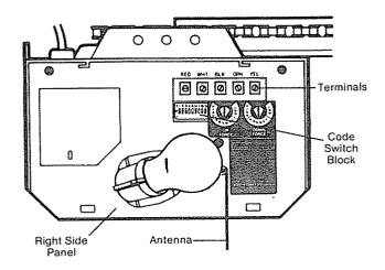
RADIO CONTROLS consist of a transmitter and a receiver. The transmitter sends a coded signal from outside the garage. The receiver is fastened to the right side panel of the door opener. It receives the transmitted signal and starts the door opener.
